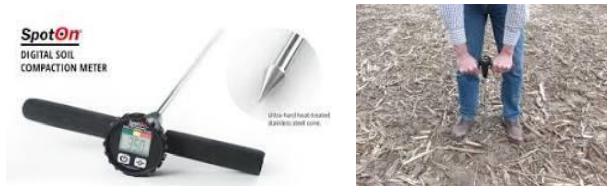
Fig. 4. Example of digital soil compaction meter and its use in a field.
