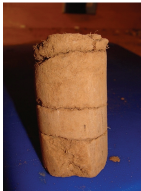
Figure 1: An excessively compacted soil core (4 inches) collected in July from a grazeout wheat pasture.
