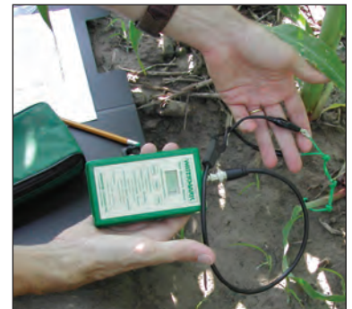
Figure 4. Using handheld meter for Watermark® sensor.
