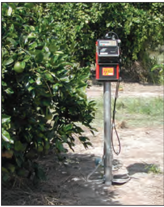
Figure 12. Neutron probe used at a citrus orchard.
