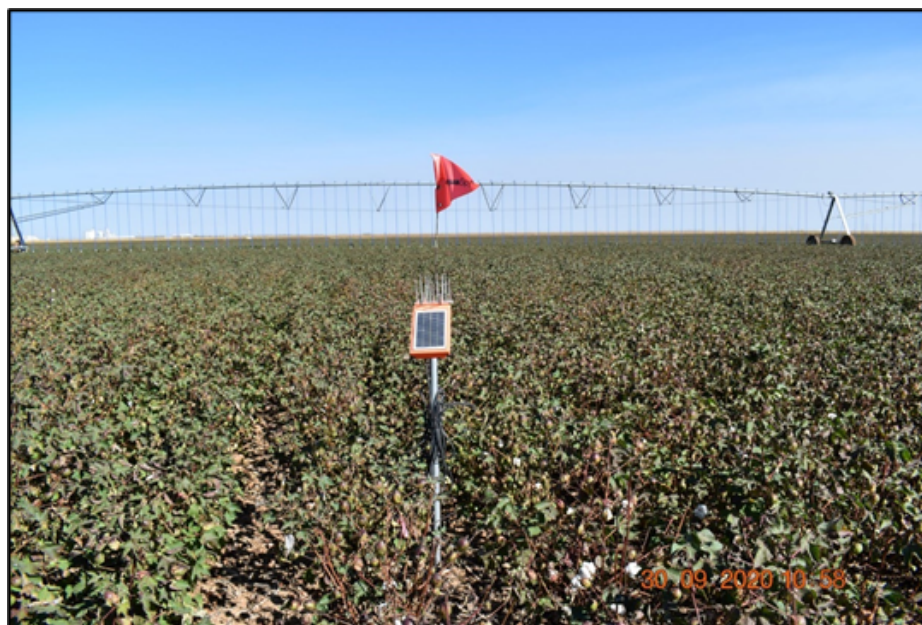
Plate 4. Electronic-based soil moisture sensors installed before planting and used to monitor the status of moisture season long and beyond at interval depths in the soil profile. North Plains Groundwater Conservation District Farm, Moore County, 2020.
