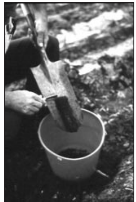
Figure 1. Soil sampling is the most important step in soil testing. Above is an example of a 1 x 1 x 6-inch core taken with a spade.
